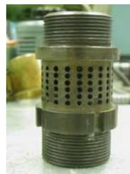
A perforated barrel (left) is used on the press (above) to allow oil to be separated from the soybeans.
