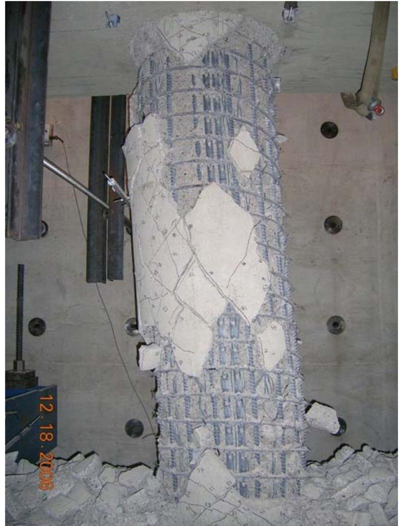
**Photograph of half-scale column test**
