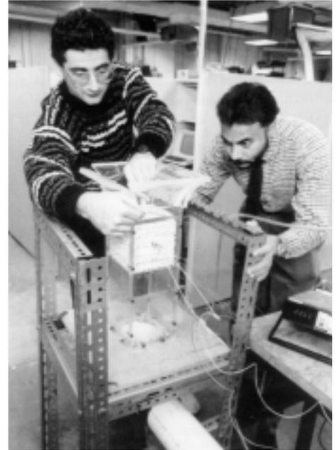
Apparatus for determining the convection heat transfer coefficient for air flow through tubes imbedded in ceramic particles. This investigation provides an understanding of fundamental mechanism occurring in packed-bed type combustion heat exchangers (1991).
