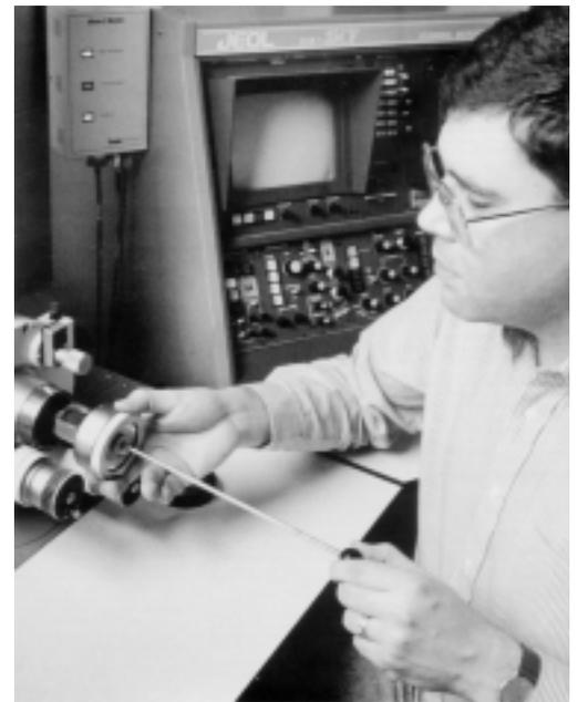
Scanning electron microscope (SEM) for examining dendritic structure and measuring solute distribution is used to understand the relationship between microscopic and macroscopic transport processes during metal alloy solidification (1990).
