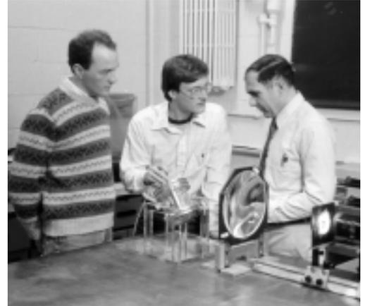
A flow visualization experiment that will consider the effect of orientation relative to gravity on the solidification of crystals in annular cavities used for thermal management of very large scale integration (VLSI) circuits (1986).
