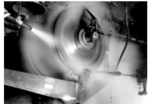
Water jet cooling of railway car wheel.
