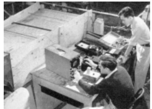
Heat loss from transmission lines are measured using wind velocities up to 60 miles per hour and currents up to 100 amperes (1950).
